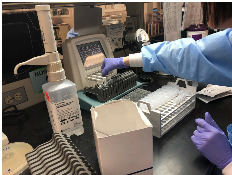
Fig 3. Inserting AST GP67 cartridges (VITEK 2) into tubes containing pellets resuspended in 0.45% sterile saline.
